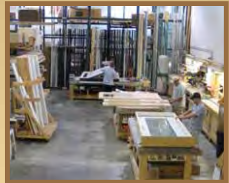
Assembly Area For Multi-Panel Entrance Systems
